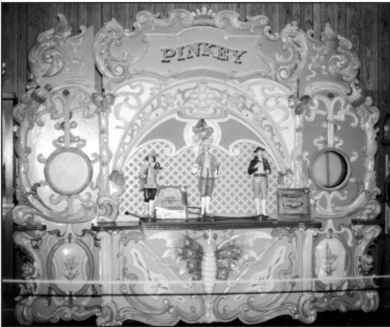
Figure 35. Paul Eakins bestowed the name Pinkey on the Luna Park-Cleveland organ that later served at Puritas Springs Park. The chassis was altered from 65 to 87-key roll format. Author's photograph.
