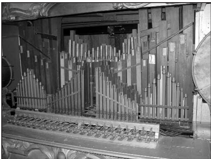
Figure 39. The characteristic pipework of a 65-key Gavioli is observed in this contemporary view of the first Gavioli that served with PTC carousel #21. Art Reblitz photograph.
